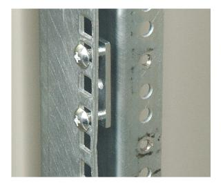
**7** Insert the slotted foot at the back of each cabinet rail between the nut bar and the post, then tighten the screws.
